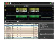
USB serial trigger and decode provides powerful time-correlated views of waveforms and symbols to the bit level, making it easy to isolate communication faults to logic or analog sources.
