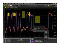
The DDR2 compliance test application provides a fast and easy way to test, debug and characterize your DDR2 designs and includes crucial measurements, such as eye-diagram, mask testing and ringing.
