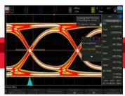
New performance standard. Get both portability and performance with surprisingly low starting prices and standard hardware bandwidth limit control, achieving a noise floor of 210 uVrms at 1 mV/div (6 GHz) and 115 uVrms at 1 mV/div (1 GHz).
