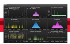
Get deep insight into your digital designs. EZJIT Plus features two methods to properly separate the jitter into random and deterministic components. If you have bounded uncorrelated jitter, simply use Keysight's new tail-fit algorithm; otherwise Keysight's spectral method and 75 fs of sample clock jitter ensure the most accurate measurement.
