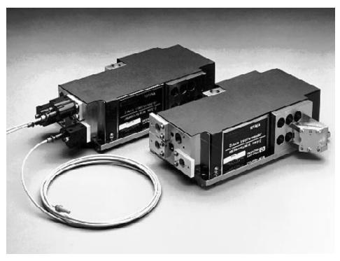
The Keysight 10735A and 10736A replace three interferometers and multiple beam benders and beam splitters with a rigid, high-performance package.
